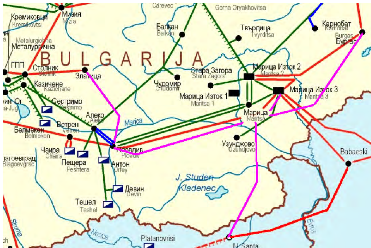
FIG. 93 REINFORCEMENTS OF THE SOUTH PART OF THE 400kV BULGARIAN NETWORK
